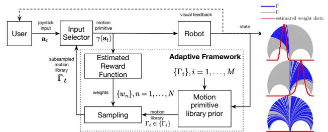
Figure 1: Left: System diagram of the proposed adaptive framework. Right: a graphical representation of the algorithm at time 0, 50, and 120 from bottom to top. The available set of the motion primitive to the user (blue) is sampled based on the inferred distribution (red) from the underlying dense set of motion primitives (grey).
