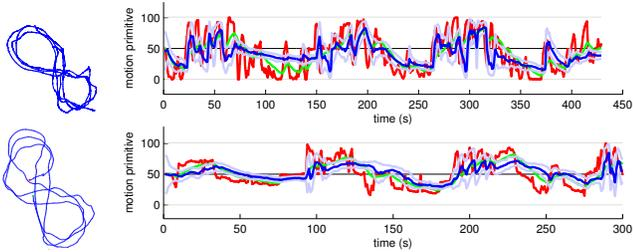
Figure 2: Comparison of simulation (top) vs. flight (bottom) results. Odometry (left) and selected motions (right) for each MPL containing 101 motion primitives. Red: actual input. Green: low-pass filter input. Blue: mean of predicted distribution with light blue highlighting upper and lower bounds based on the covariance.
